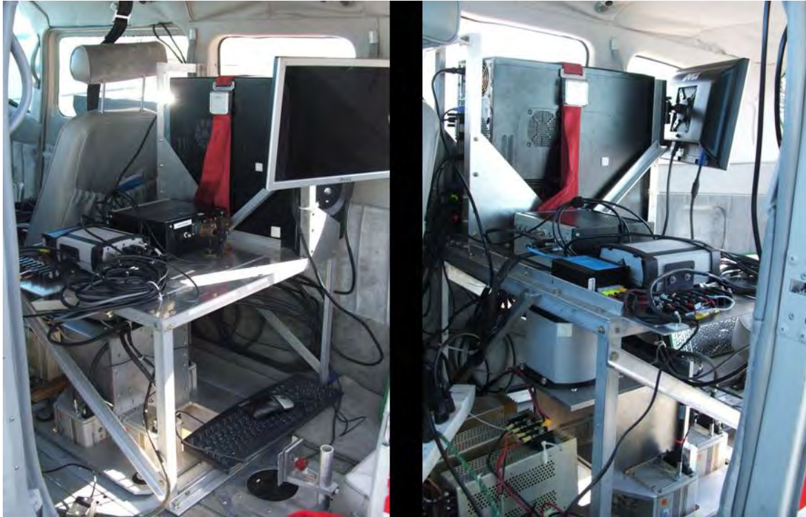
Figure 1. Details of the USU airborne multispectral remote sensing system and LASSI Lidar system installed on the USU Cessna TP206 remote sensing aircraft.
