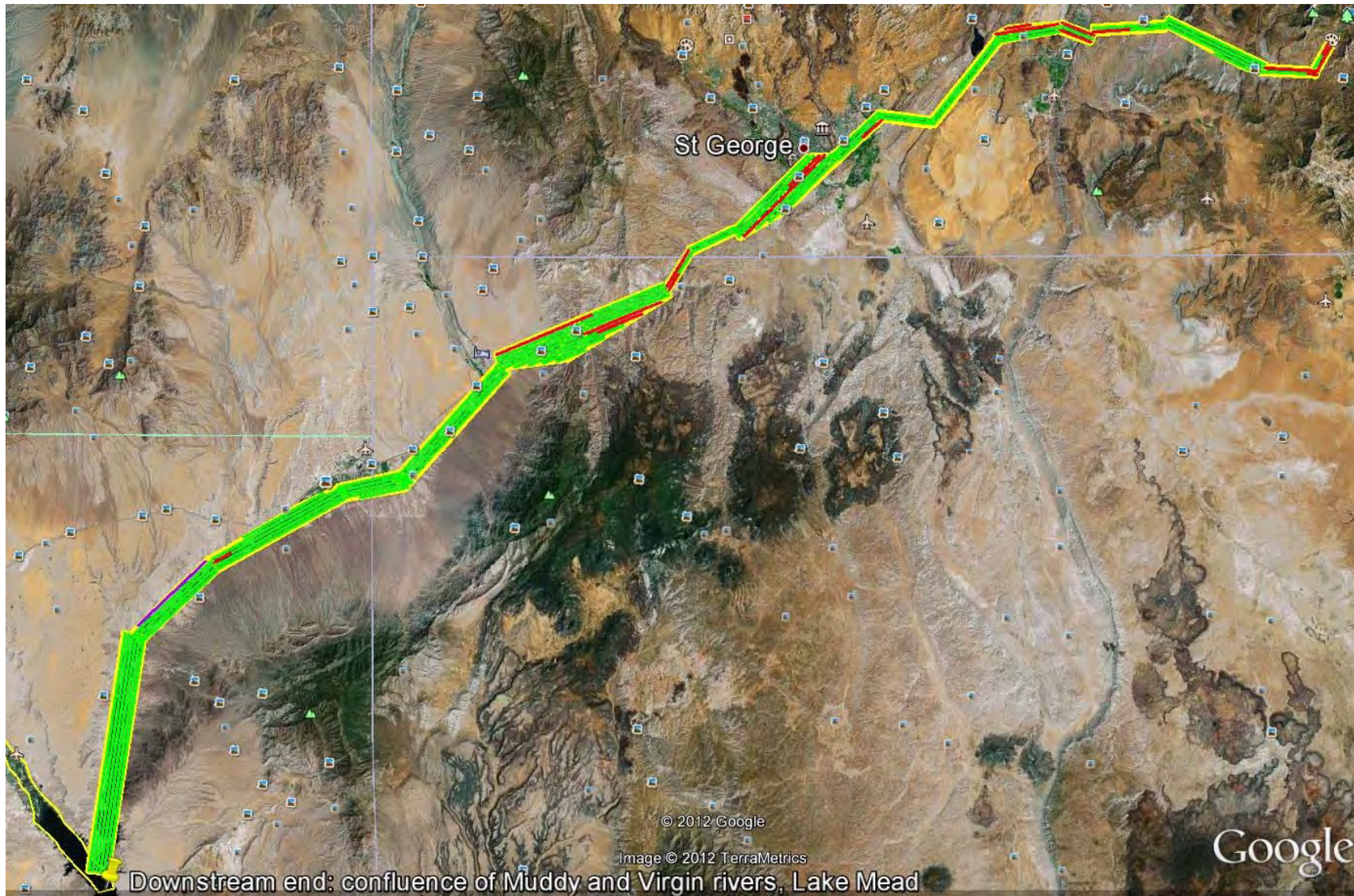
Figure 2. Schematic of the flight lines flown during the data acquisition flights. Red lines indicate missing multispectral imagery.
